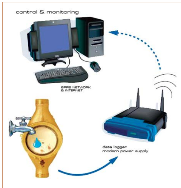
Figure 1. Typical Smart Water Meter Set-up.
